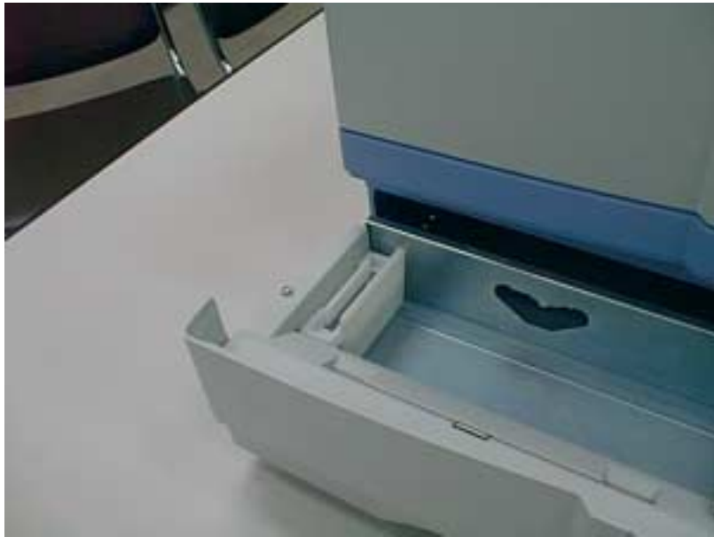
3) Lock the card push plate. Photo2-3
