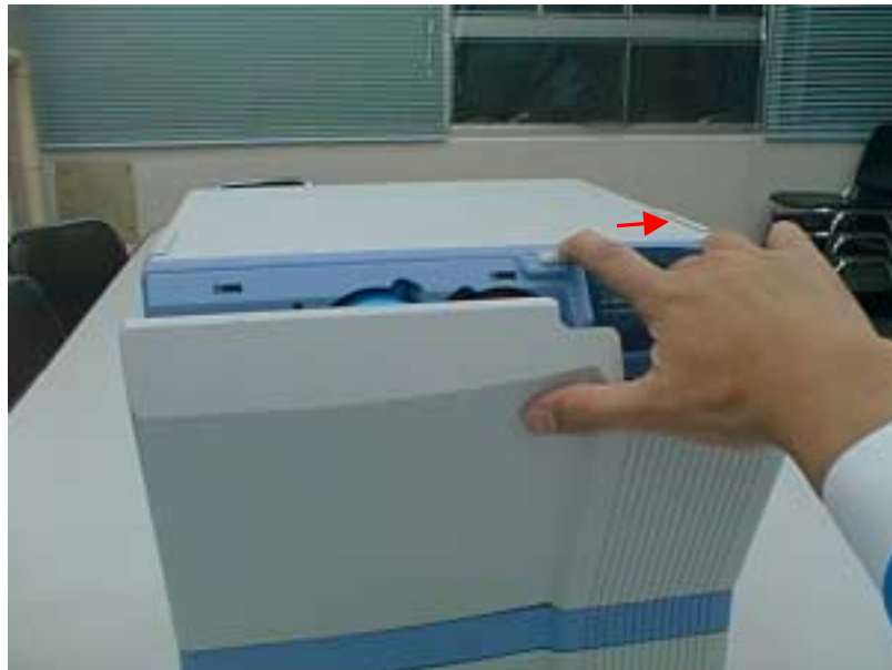
1) Slide the door lock lever. Photo3-1
