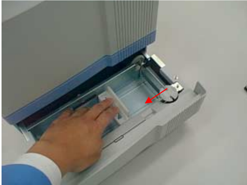
2) Move the card push plate. Photo2-2
