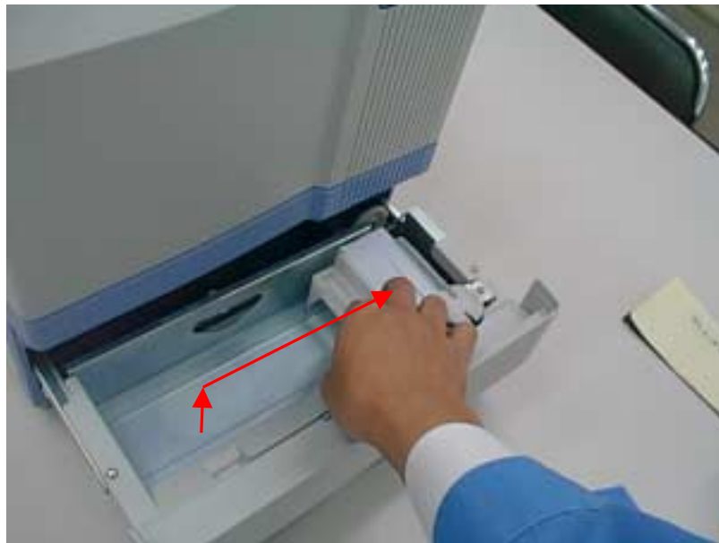
5) Lift up the card push plate, and hold the cards. Photo2-5
